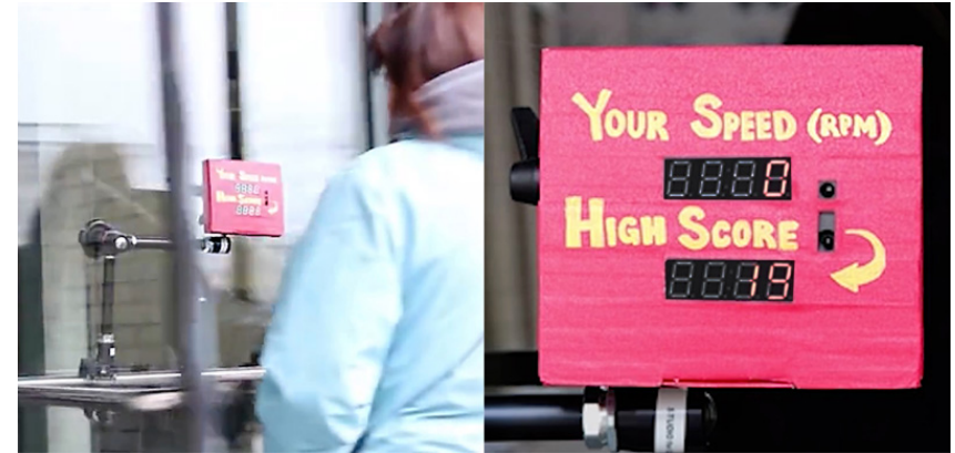
125. Michelle Ma's Revolving Games (2013), another student project, measures the speed of a revolving door with an accelerometer, then displays the high score on an LED. Ma's game encourages risk-taking in an otherwise quotidian setting.
