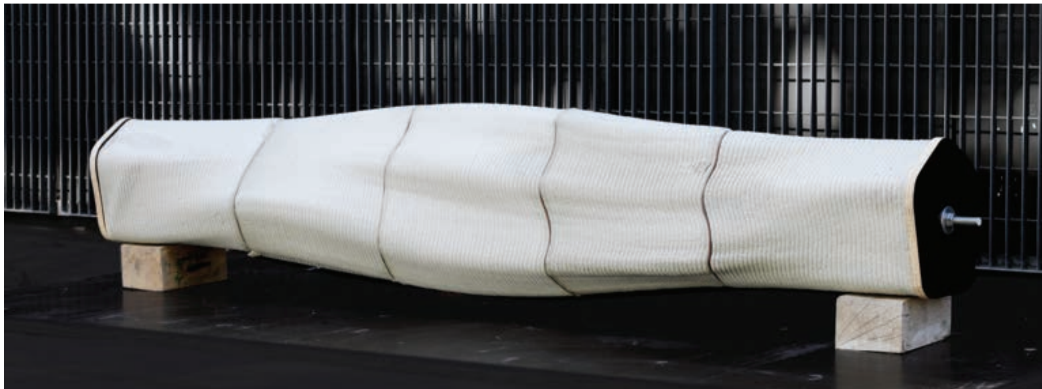
Printed prototype beam, designed and fabricated using the tool.
