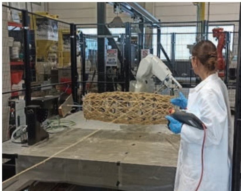
Winding of rope impregnated with resin.
